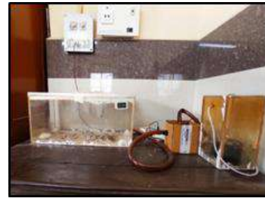
Figure: Cigarette smoke exposure chamber
